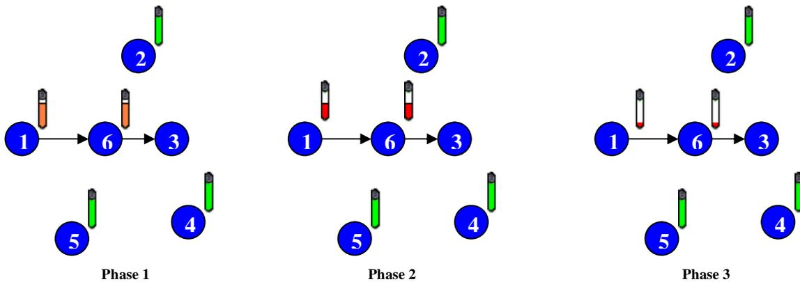
Figure 1. Battery Status without Power Aware Routing following only Shortest Path Algorithm
