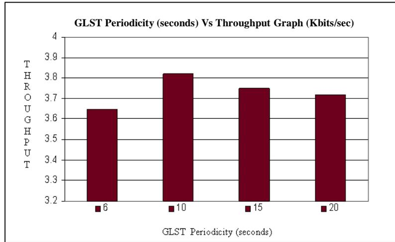
Figure 6. GLST Periodicity vs Throughput in Mobile scenario
