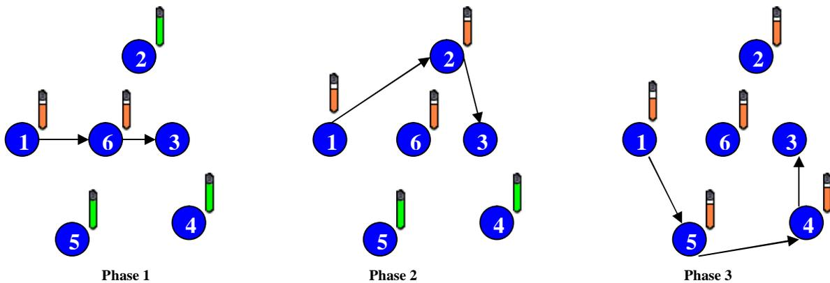
Figure 2. Battery Status with Power Aware Routing together with Shortest Path Algorithm
