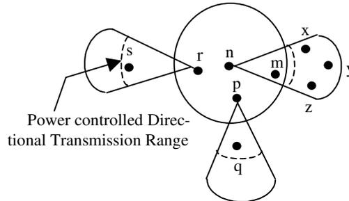
**Fig. 1.** Improving SDMA efficiency with Directional Antenna and power-controlled Directional Transmission
