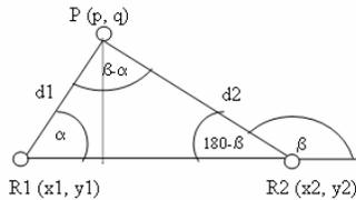
Figure 3. Illustration of Coordinate calculation using 2 reference nodes
