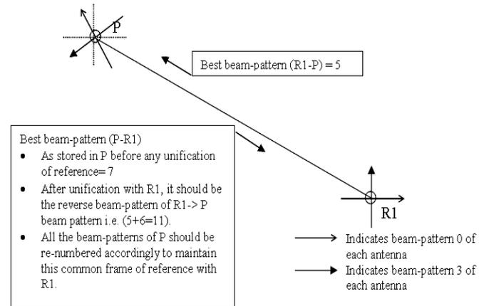
Figure 4. Illustration of Unification of orientation of antenna using reference
