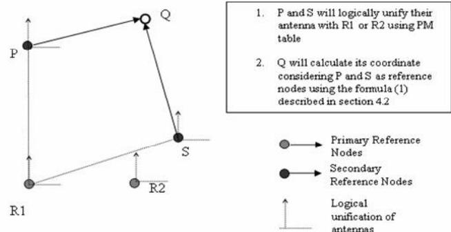
Figure 5. Location estimation by node Q using reference nodes P and S
