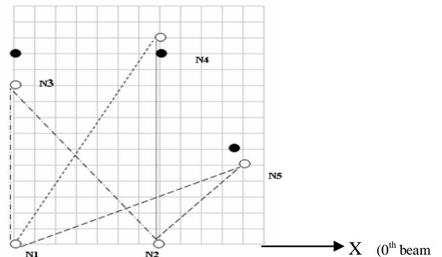
Figure 6. Single-hop location estimations of N3, N4 and N5 with two reference nodes N1 and N2
