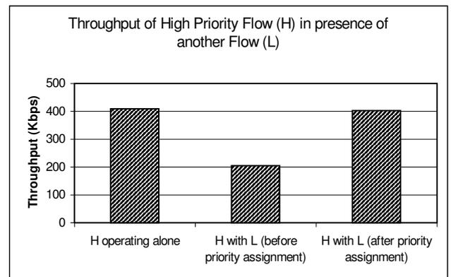
Figure 5. Throughput of a High Priority Flow (H) in presence of another Flow (L) with and without Priority Scheme
