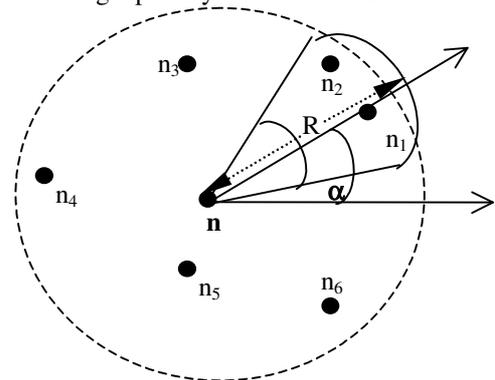
Figure 2. Transmission Zone $_n(\alpha, \beta, R)$  and omni-directional transmission range [in dotted lines] showing directional and omni-directional neighbors
