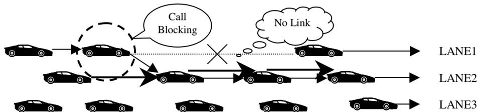
Figure 1(d). Initiation of a high priority flow from a car in LANE2 handling an existing low priority communication forces the low priority flow to block itself due to the absence of any other alternative path
