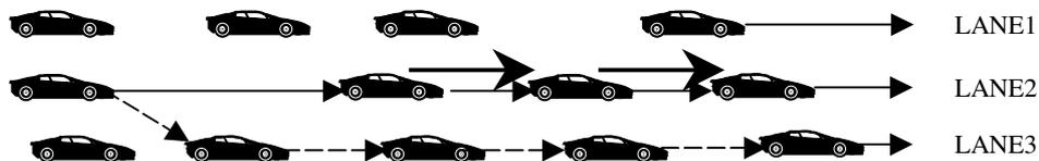
Figure 1(c). Initiation of a high priority flow from a car in LANE2 handling an existing low priority communication causes the low priority flow to take a diverse route along LANE3.
