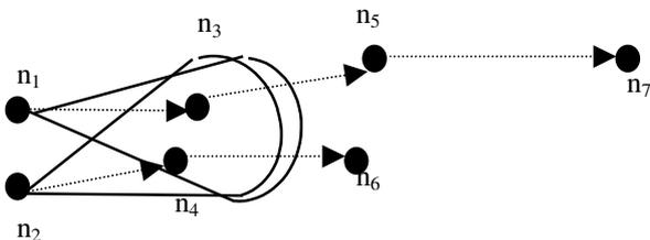
Figure 3. Route Coupling causes contention in wireless medium
