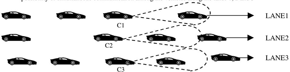
Figure 1(b). Non-overlapping transmission-zones of cars C1, C2 and C3 using directional antenna enhances the possibility of simultaneous communication among the vehicles along the lanes 1, 2 and 3
