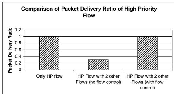
Figure 5: Comparison of Packet Delivery Ratio of High Priority Flow
