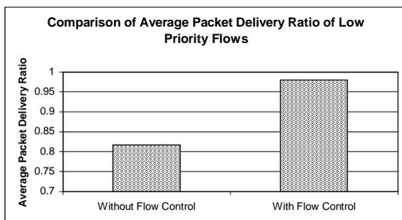
Figure 7: Comparison of Average Packet Delivery Ratio of Low Priority Flows
