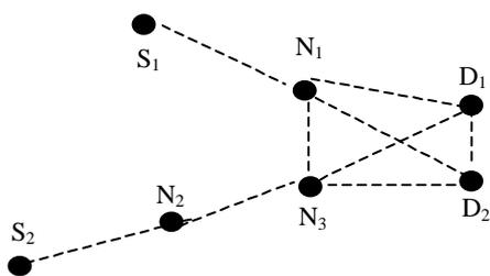
Figure 1: Using omni-directional antenna Low Priority Flow ( $S_2$ - $D_2$ ) is disturbing High Priority Flow ( $S_1$ - $D_1$ ).
