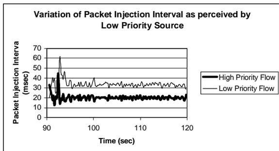
Figure 3: Variation of Packet Injection Interval of Low Priority Flow based on the perceived Packet Arrival Interval of High Priority Flow at Low Priority Source
