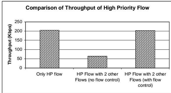
Figure 4: Comparison of Throughput of High Priority Flow
