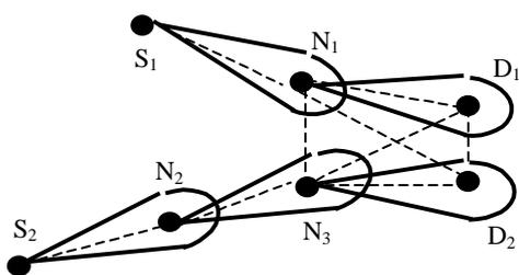
Figure 2: Using directional antenna Low Priority Flow ( $S_2$ - $D_2$ ) can coexist with High Priority Flow ( $S_1$ - $D_1$ ).
