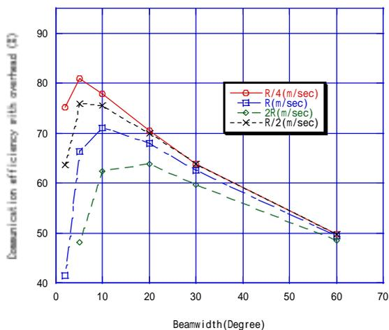
Fig.6: Communication efficiency with overhead (n=400)
