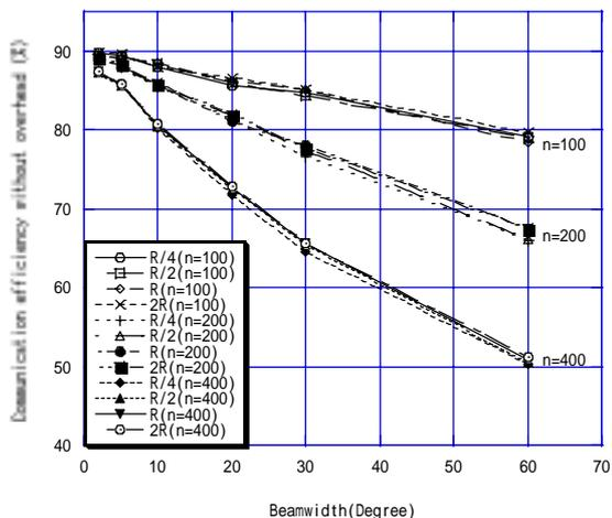
Fig.3: Communication efficiency without overhead
