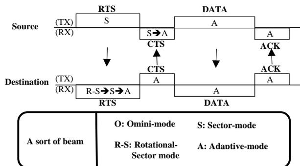
Figure 1: Example of antenna modes of 4-way-handshake in MAC\_2
