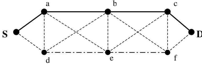
Fig. 1. . Two node-disjoint path with  $\eta = 9$
