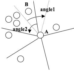
Figure 3: Optimization of the transmission angle: transmission within the angle1 is better than transmission within angle2
