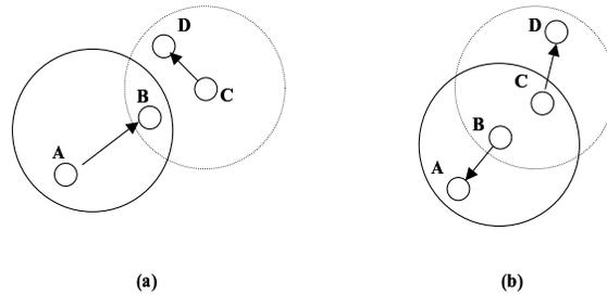
Figure 1: Examples of Hidden (a) and Exposed (b) Node problems. The circles indicate the radio transmission ranges
