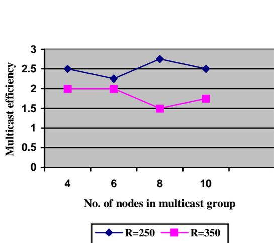
Figure 2. Multicast efficiency for different number of nodes in multicast group at different transmission range
