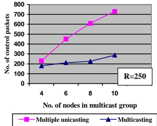
Figure 1. Number of control packets generated for different number of nodes in multicast group at different transmission range ( R ).
