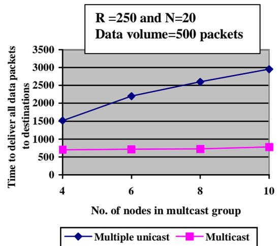
Figure 3. Time to deliver all data packets to destinations with multicast and multiple unicast
