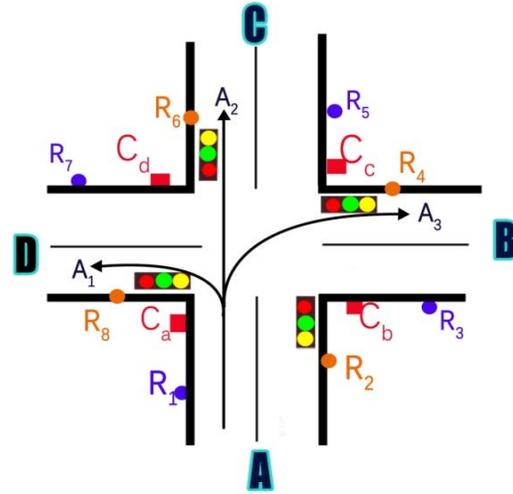
Figure 1. Model junction with RFID devices
