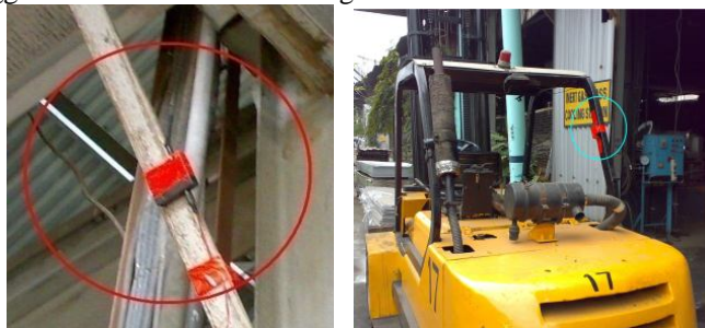
Fig. 2(a). Placement of a mesh router; 2(b). Tagged FLT.
