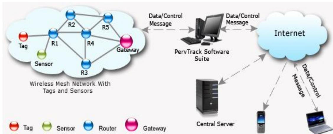
*Figure 1. A conceptual framework for Monitoring and Actuation of objects and environment through the Internet*
