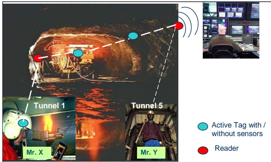
**Figure. 4.** Conceptual framework for Underground Miners' Tracking & Poisonous Gas Detection System:
