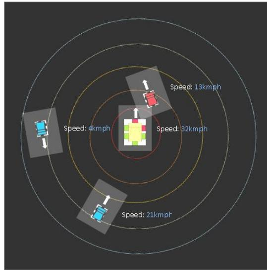
*Fig. 2. The visual display at the driver's cabin of "yellow" dumper where relative position of other dumpers in the vicinity of 300 meters are shown. The red dumper is in the collision range, as indicated by overlapping dumper shield (Early warning) and also two red dots on yellow dumper (proximity warning)*
