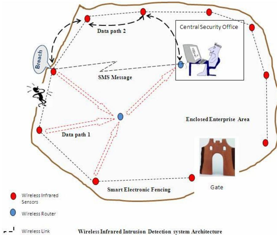
**Figure 5.** Conceptual framework for Wireless Infrared Intrusion Detection (WIID) system
