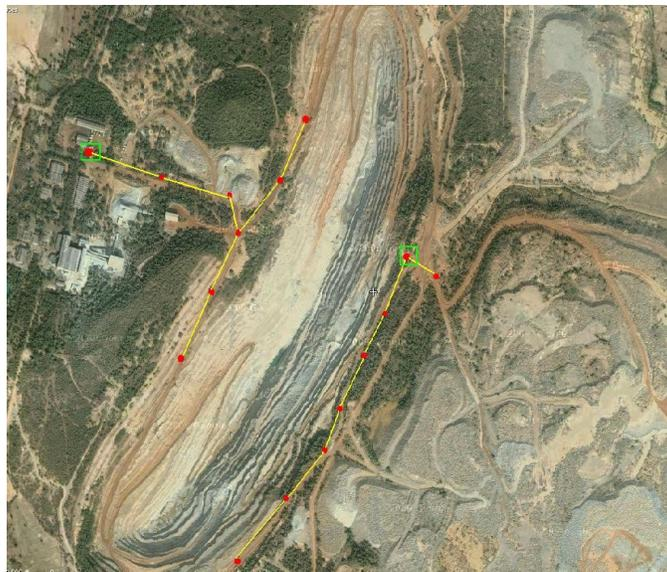
*Figure 3: Sample mining site with Wireless Mesh Network, depicted by red dots*
