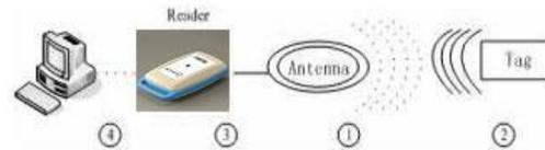
**Fig. 2 Work Process of RFID Technology**
