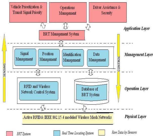
**Fig .3 Schematic Representation of System Architecture of BRT management System based on Active RFID and IEEE 802.15.4 modeled Real Time Locating System**
