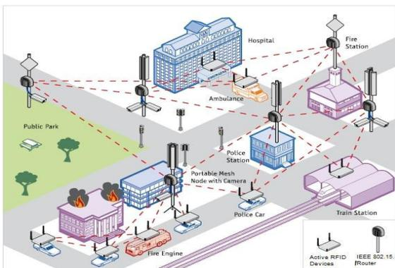
**Fig. 1 Structure of Wireless Mesh Network based on IEEE 802.15.4**
