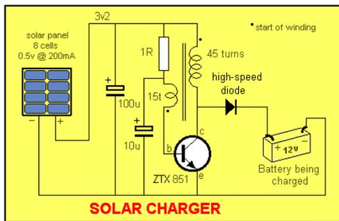
Fig 6- A simple solar battery charger circuit
