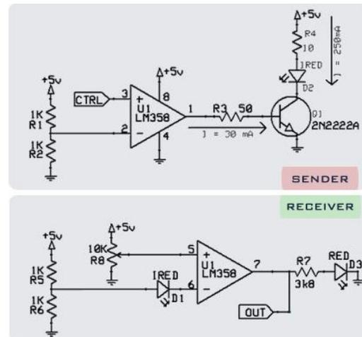
Fig 5 – Simple Transmitter and Receiver Circuit
