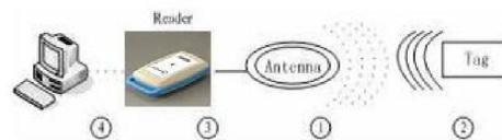
Fig.2. Work process of Radio Frequency Identification Technology
