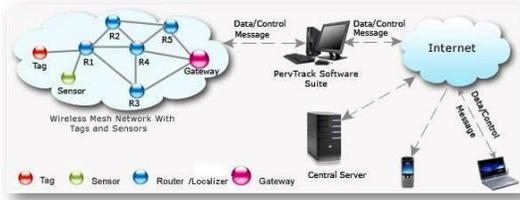
Fig.3. Structure of Wireless Mesh Network based on IEEE 802.15.4
