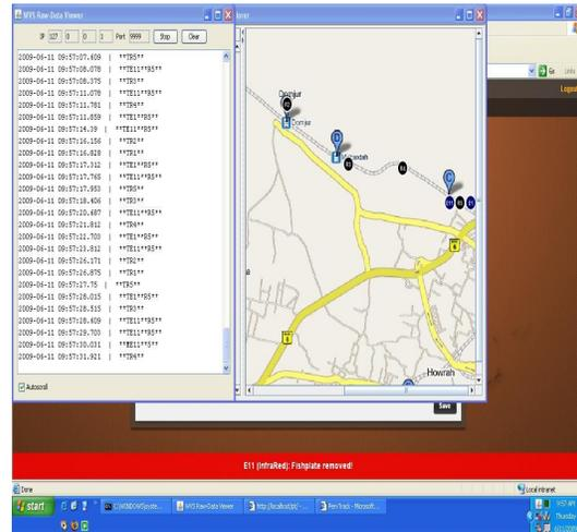
Fig. 8- Screen shot of tracking software showing warning message (in red) on removal of fish plate. Courtesy: Pervcom Consulting Pvt. Ltd.
