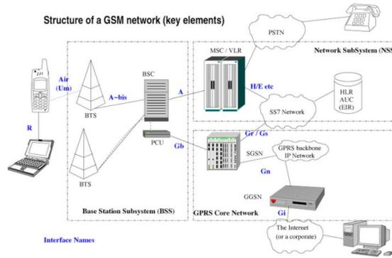
Fig. 7 Basic structure of a GSM network
