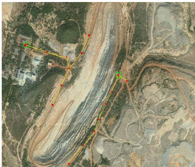
Figure 4: Sample mining site with Wireless Mesh Network deployment, depicted by red dots
