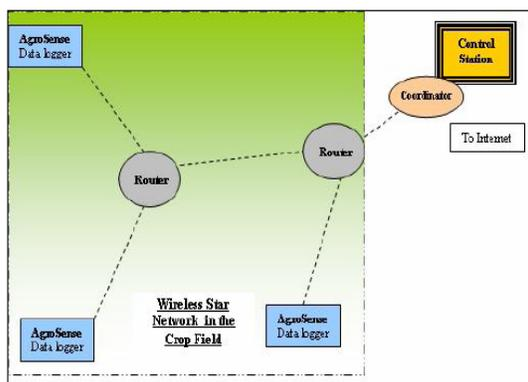
Fig. 3 AgroSense System Architecture
