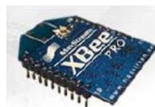
Fig. 4 XBee IEEE 802.15.4 based RF module
