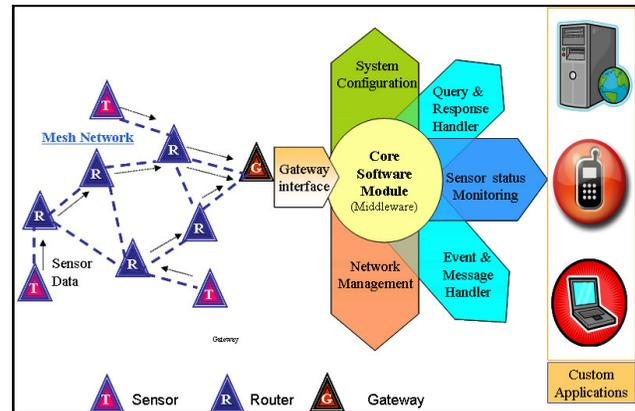
Figure 4. The system architecture
