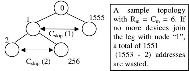
Figure 2. The address wastage problem in  $C_{skip}$
