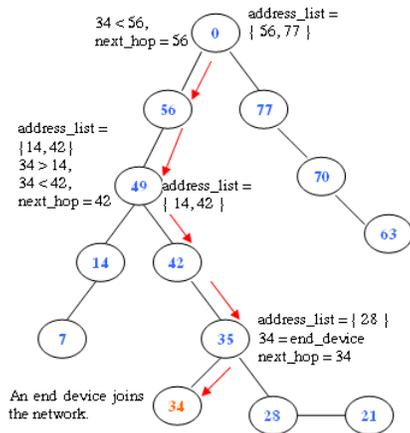
Figure 3. Addressing & Routing in the modified Hierarchical Tree.
