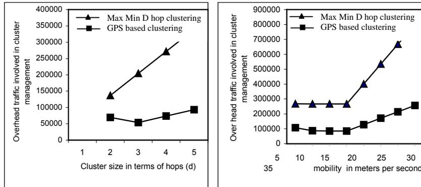
Fig. 3. Average overhead involved in cluster maintenance with a) varying cluster size
