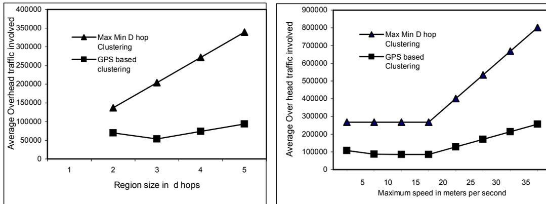
Fig. 3 Average overhead involved in cluster maintenance with a) varying cluster size b) varying node mobility.
